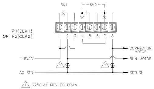
All circuits should be fused or protected by a circuit breaker (10Amp maximum)
